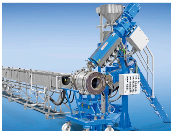
Extruder Group with Cross Head in a Sheathing Line
