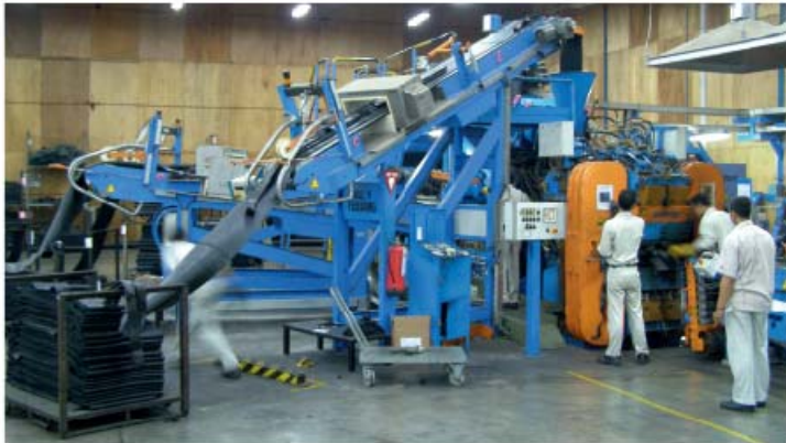
Quadruplex unit with slab feeders Cushion calender Quadruplex head with 3 extruders Rotating cross cutter as part of a wind-up system Cassette wind-up station
